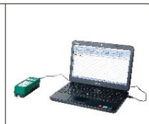
data can be output to Excel by connecting computer via bluetooth or USB cable
